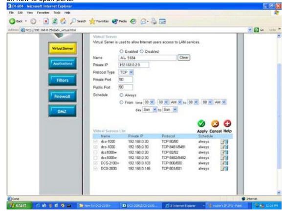
Enter valid ports in the **Virtual Server** section of your router. Please make sure to check the box on this line to enable settings. Then the device can be access from WAN by the router's WAN IP Address.
